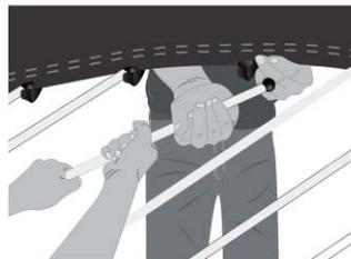
7 Inside and Outside Person: Lower the white mat rod and carefully ease it to a resting position.
