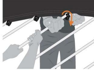
6 Inside Person: Once the ball comes to the back edge of the mat rod holder, pull the white mat rod down and out. Sometimes a forceful pull is needed to dislodge the ball from the mat rod holder.
