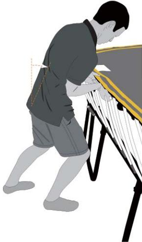
5 Outside Person: Push forward, rocking from your heels to the balls of your feet, using the weight of your body to push the white mat rod over the back edge of the mat rod holder. Keep the mat edge horizontal with your other hand.
